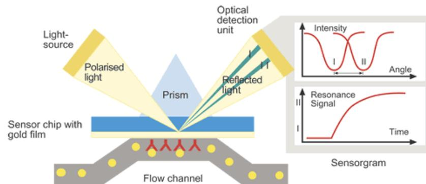
**Figure 1.** Schematic of the SPR experimental setup and representative data (sensogram) collected during SPR measurements. (<http://www.rci.rutgers.edu/~longhu/Biacore/>)
